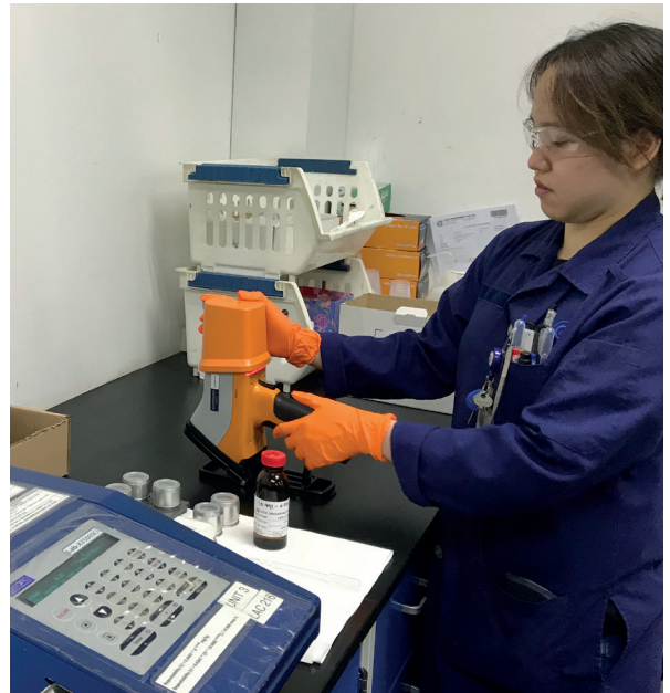
Testing bunker fuel using X-MET8000
