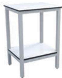
Table for furnaces, ovens and incubators. Two heights with a separation of 74 cm. Worktop made of high resistance compact phenolic resin Fundermax Resistance<sup>2</sup> soft grey, 20 mm thick. Ideal for all types of laboratories. Tube metal frame made of cold rolled steel 40 x 40 mm, with an antirust epoxy resin protection layer. With a maximum load capacity of 300 kg. Four adjustable support points to level the table. Delivered assembled. Warranty 5 years. Delivery time: 4 weeks
