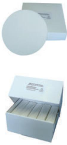
Low ash paper (max 0.06%) made of cotton fibers, used for thick and sticky liquids filtration. Surface weight 85 g/m<sup>2</sup>, pore 10 - 12 µm, thickness 200 µm. Available in flat disks and folded. Equivalence: Whatman 4
