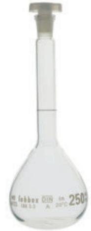
**VOLUMETRIC FLASK CLASS A WITH PLASTIC STOPPER**
