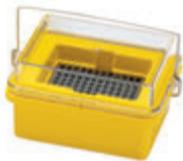
This cooler is designed in polycarbonate (PC) to protect enzymes and solutions by maintaining them at temperatures between -20 °C and -15 °C up to 2 hours during sample preparations on the bench. Base is filled with non-toxic gel. Yellow color. The aluminum block has 96 (8 x 12) wells to hold tubes, strips or plates of 0,2ml. Freeze for 24hrs at -20 °C to -25 °C prior to use
