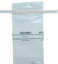
Made of highly resistant polyethylene (FDA-approved). Easy-to-close bags with puncture-proof tabs for protection from possible damage due to wire-end punctures. Ideal for chlorinated water samples, with thiosulfate tablets (10 mg / 100 ml), to perform bacterial testing. Maximum bag mouth opening and write-on strip and volume markings for measurements. DNase, RNase and pyrogen free. Free sterilization certificate available on the website
