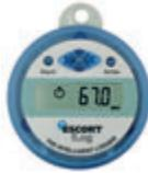
32000 readings. Temperature measuring range -40 °C to 70 °C, resolution 0.1 °C and accuracy  $\pm 0.3$  °C. Humidity measuring range 2% to 98%, resolution 0.1% and accuracy  $\pm 3\%$ . LCD displays the minimum, maximum, average and time out of specifications. Data can be downloaded to PC with LOGH-A01-001 (not included) and managed with Console Plus software. IP51. Power supply: 3,6V Lithium battery LS14250 1/2AA. Warranty 2 years
