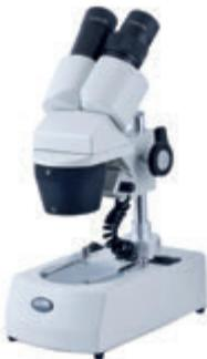
Binocular head 45° inclined. Widefield WF10X/20mm eyepieces. Turret-type magnification changer with 2X and 4X objectives. Incident and transmitted (according to model) tungsten 12V/10W or LED 20 mA, 3.5V, 70 mW illumination. Dust cover included. Supply 220-240 V (CE). Warranty 5 years on optical and mechanical components. Delivery time 2-3 weeks
