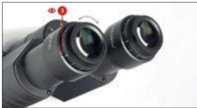
3- Then look through the eyepiece on the left with your left eye. Use the dioptre's adjustment ring to focus to focus the sample until the image is sharp
