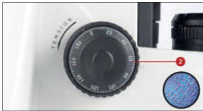
2 - Focus the image by using the fine and or coarse focusing adjustment knobs until the image of the specimen is sharp
