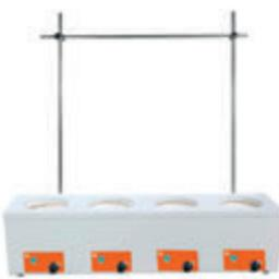
Electronic temperature regulation for each position. Maximum mantle temperature of 450°C at the surface (the maximum temperature reached by the liquid is lower due to heat loss). Continuous operation. Fast, uniform and safety temperature regulation. Featured by anti-corrosion, age-resistant, durable and safe. Easy to operate. Includes aluminum rod and retort clamp for montages. 220V/50Hz. Warranty 2 years
