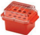
Designed in PC to keep reagents and enzymes cool. Suitable for a multitude of centrifuge tubes. Red color. Capacity of 12 tubes of up to 15 ml, array of 3 x 4. Protects samples from temperature fluctuations. The base is filled with non-toxic gel. Will maintain temperature approximately for 1 hour on the bench. Freeze for 24 hours at -5°C to -10 °C prior to use
